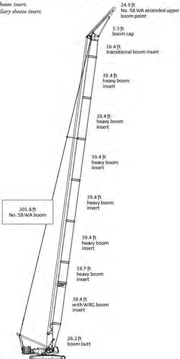
**No. 58 WA boom with BRS combinations with 24.9 ft extended upper boom point**
